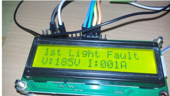
Fig.4.(b) LCD display of fault in control room.
