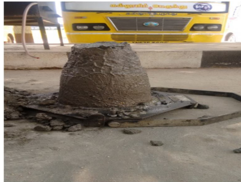
Fig: 1 Slump Cone Test
