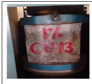
Fig 2 Compressive Strength Test
