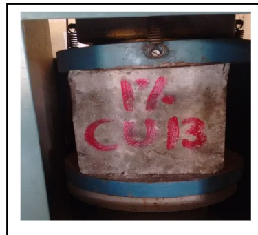
Fig 2 Compressive Strength Test
