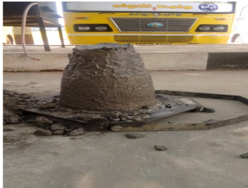
Fig: 1 Slump Cone Test
