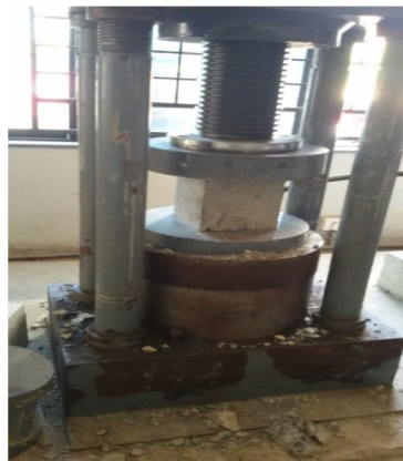
Fig.2 Compression Strength Test Set up
