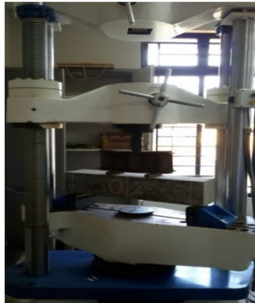
Fig. 4 Flexural Strength Test Set up
