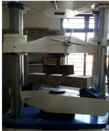
Fig. 4 Flexural Strength Test Set up
