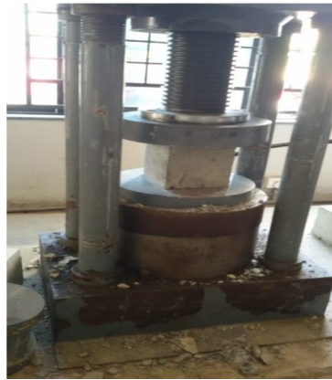
Fig.2 Compression Strength Test Set up
