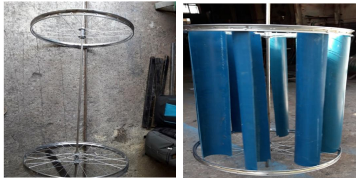
Fig 5 Mounting of shaft & Turbine blades
