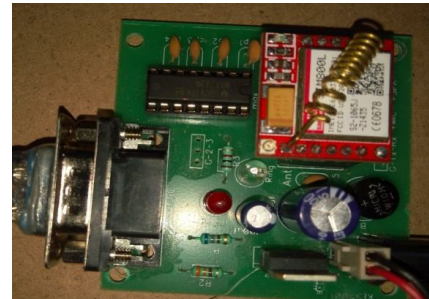
fig 5b:-DESIGNED AND FABRICATED GSM MODEM
