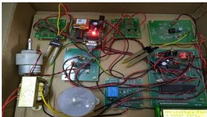
FIG (4.1): circuit for agriculture field motor control system based on IOT
