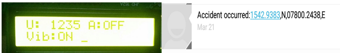
Fig9. LCD displaying vibration sensor is on and alert message sent to mobile
