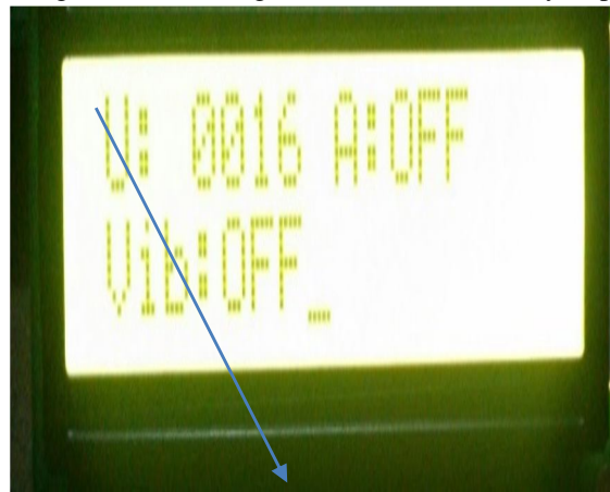
Fig11. When obstacle is detected ahead speed is minimum
