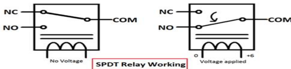
Fig.2.Working of Relay
