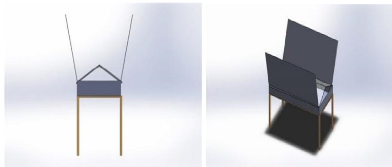
Fig. 4 Solar still (a) Front view and (b) Isometric view
