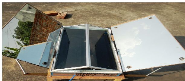
Fig. 5 Double slope solar still - working model construction Table.I Experimental Output Values
