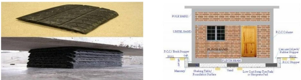
Figure 2: Use of Waste Tire Pads
