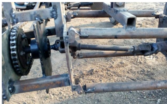
Figure 2.3: Power Transmission system
