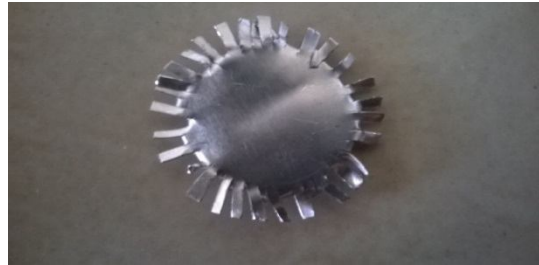
Fig 2 fabricated serrated fin with above dimensions.
