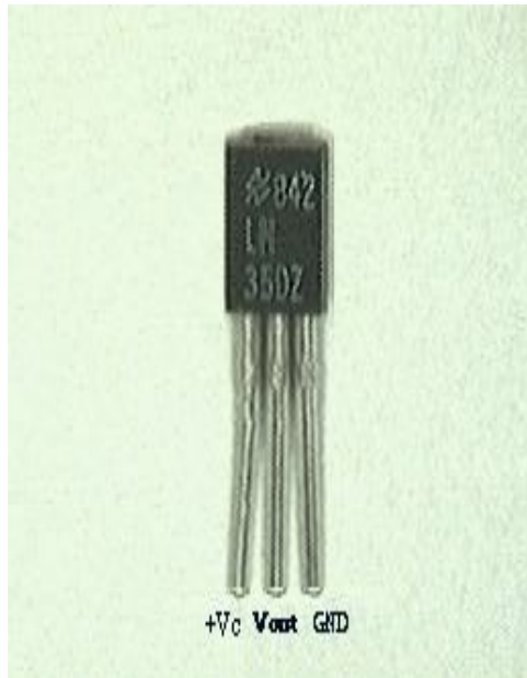
Figure 4 Temperature sensor device
