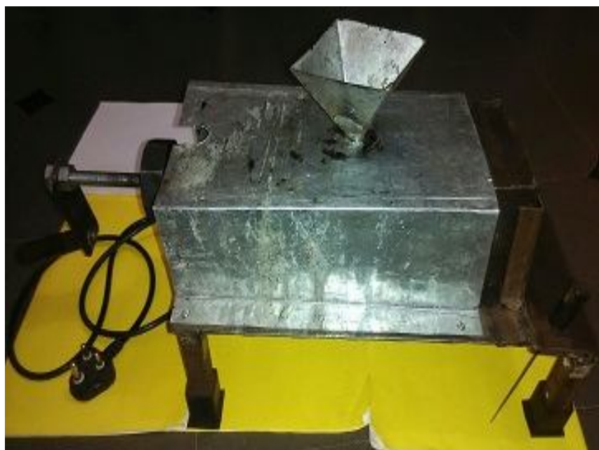
Figure3 : Design and Developed Mini Injection molding machine.
