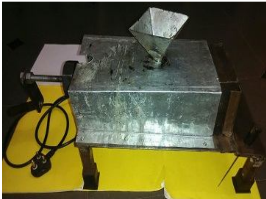
Figure3 : Design and Developed Mini Injection molding machine.
