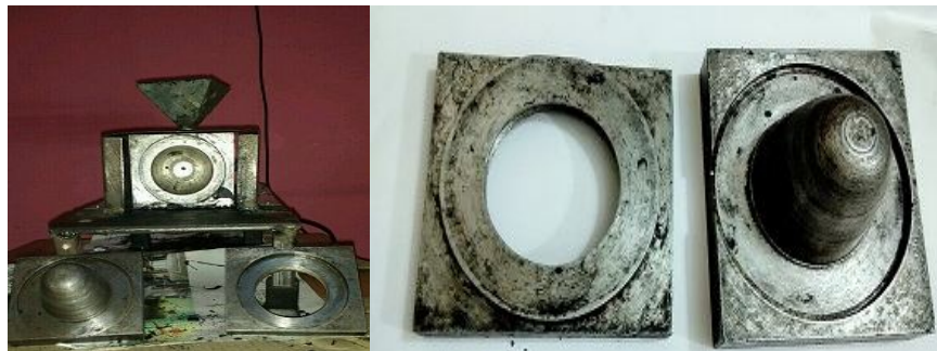
Figure2 : Mould used in injection molding machine
