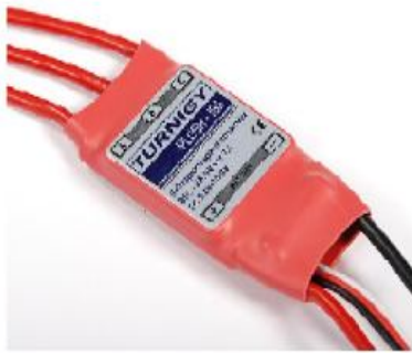
Fig.6. ESC circuit used in snapper
