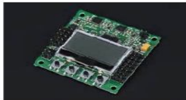
Fig.9. Flight Controller circuit used in snapper
