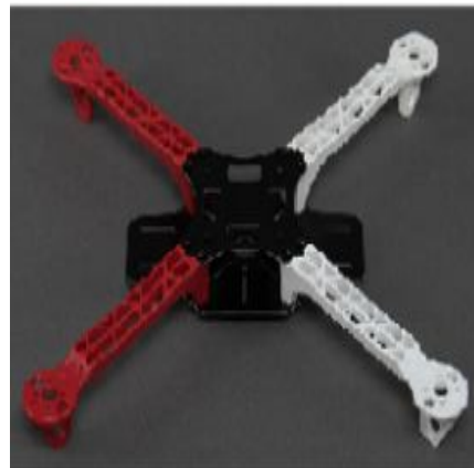
Fig.3. frame of snapper
