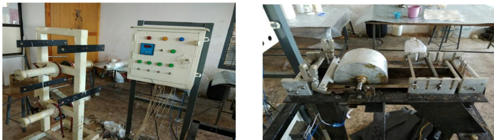
Fig. 1: Creel Stand and Resin Bath
