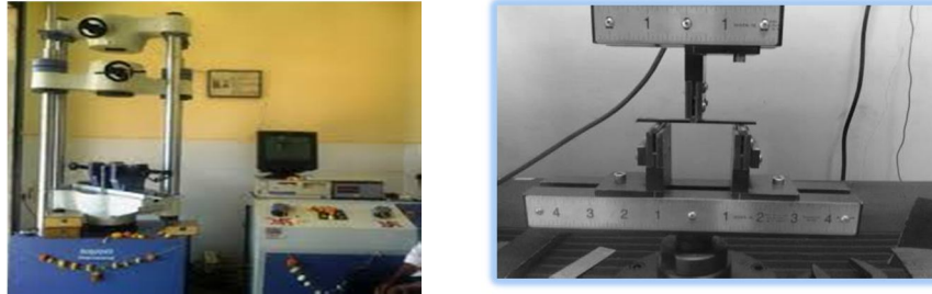
Fig. 3: UTM and 3Point Bend Test
