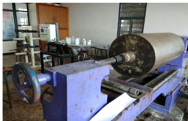
Fig. 2: Filament Winding Process
