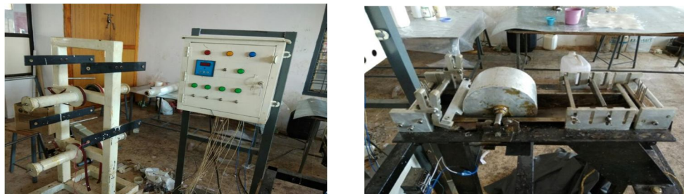
Fig. 1: Creel Stand and Resin Bath
