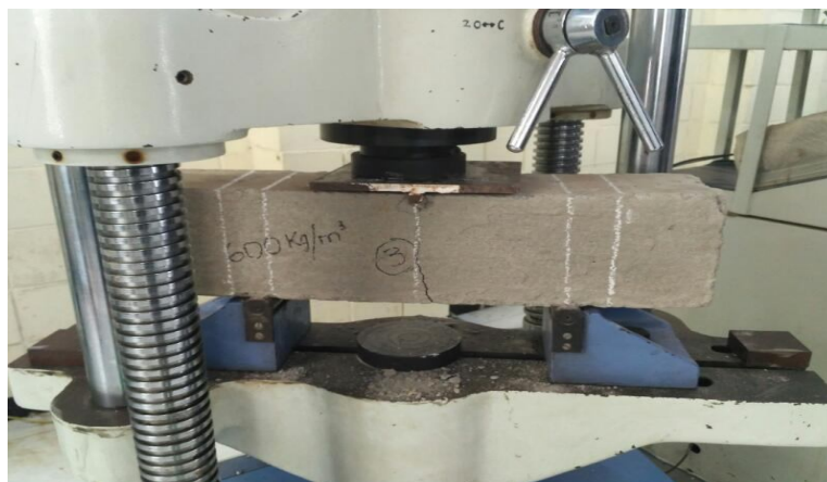
Fig.8 Flexure test setup
