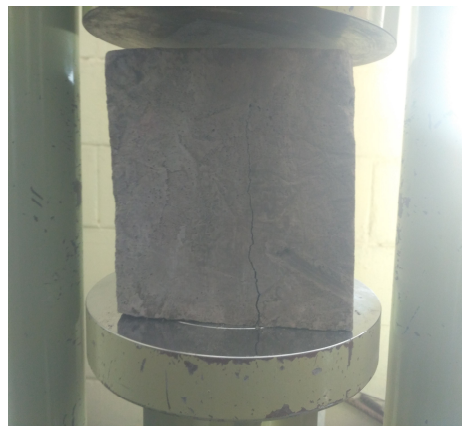
Fig.6 Compressive Strength Test
