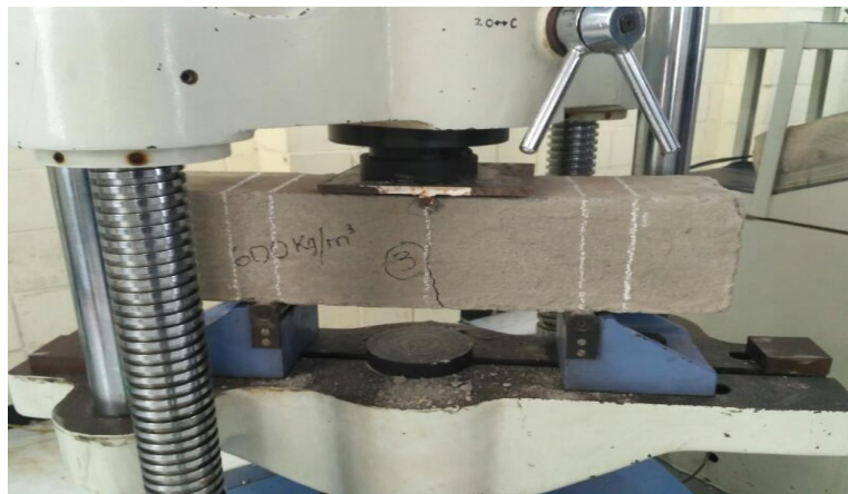
Fig.8 Flexure test setup
