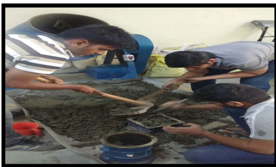
Figure 6. Casting of Specimens
