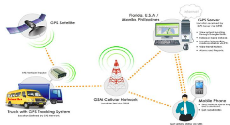
Figure 5: GPS tracking system architecture
