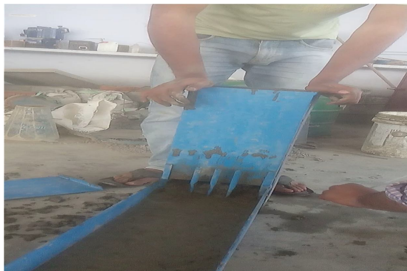
L-box test for SCC
