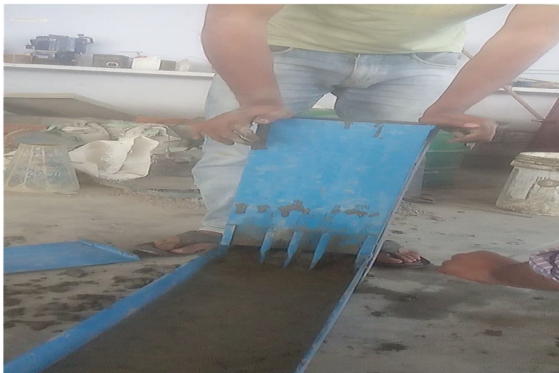
L-box test for SCC
