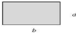
Figure 4 Cross-section of the Cantilever Beam
