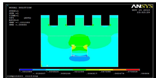
Fig. 4 Contours of heat flux using three fins for Copper processor
