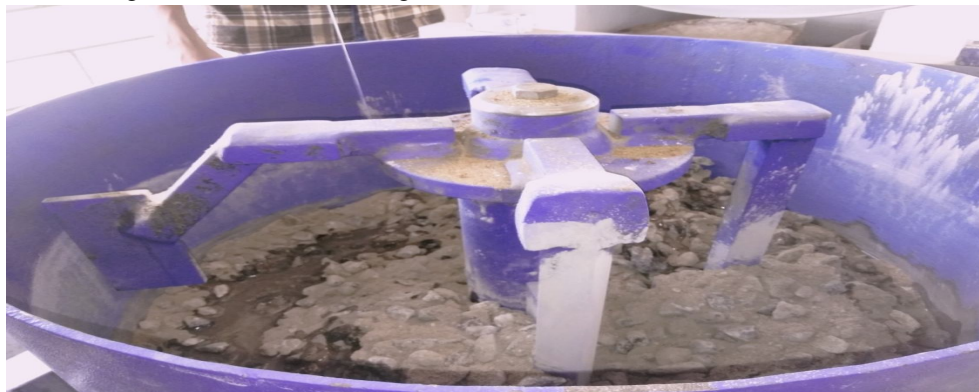
Fig. 2 Pan mixer user for mixing geopolymer concrete
