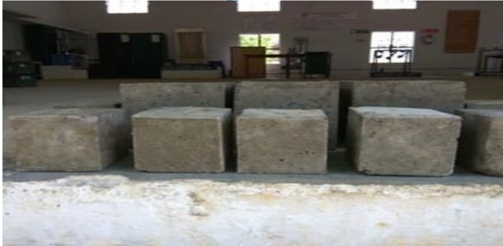
Fig. 3 100mm geopolymer cubes after demoulding
