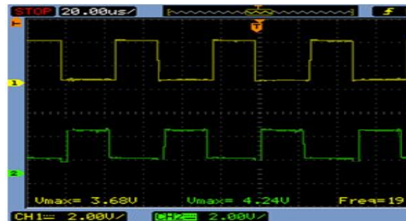
Fig. 14 Complementary pulses to the DC/AC converter
