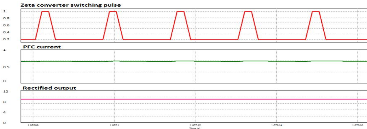
Fig. 10 Pulse waveforms of Zeta converter and rectified output.
