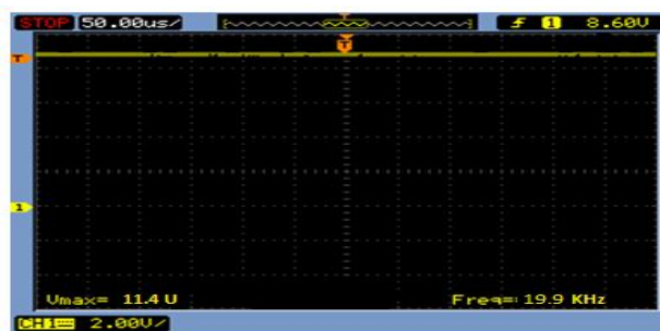
Fig. 15 Load voltage of 12 V
