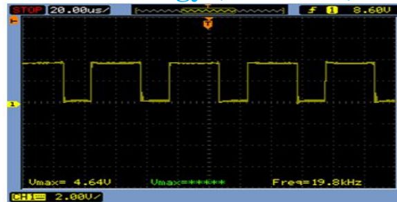
Fig. 13 Mode 2 operation of ZETA converter.
