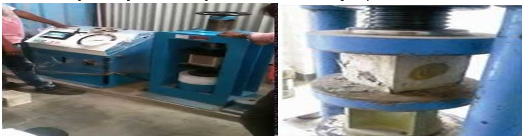
Fig 3.2 Compressive Strength Test of Cube
