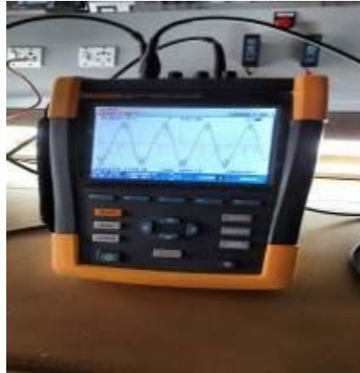
Fig.3.Measurement of Total Harmonic Distortion
