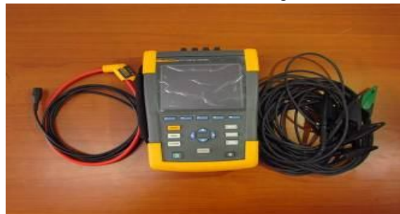
Fig.2. Flukemeter for Power quality indices measurement
