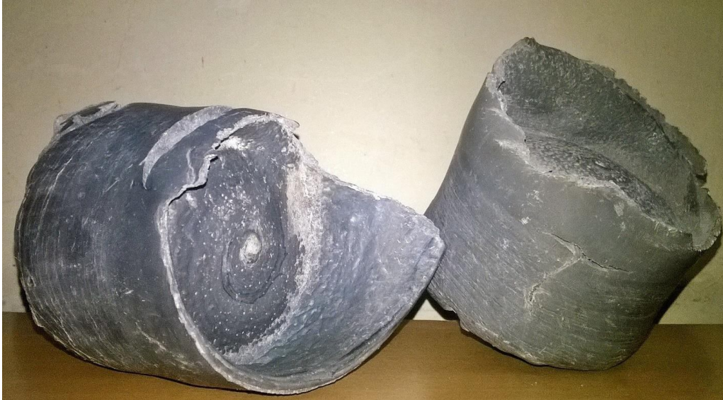
Figure1. Jali Gulla Material ( Solid Cylinder of Waste Polymer )
