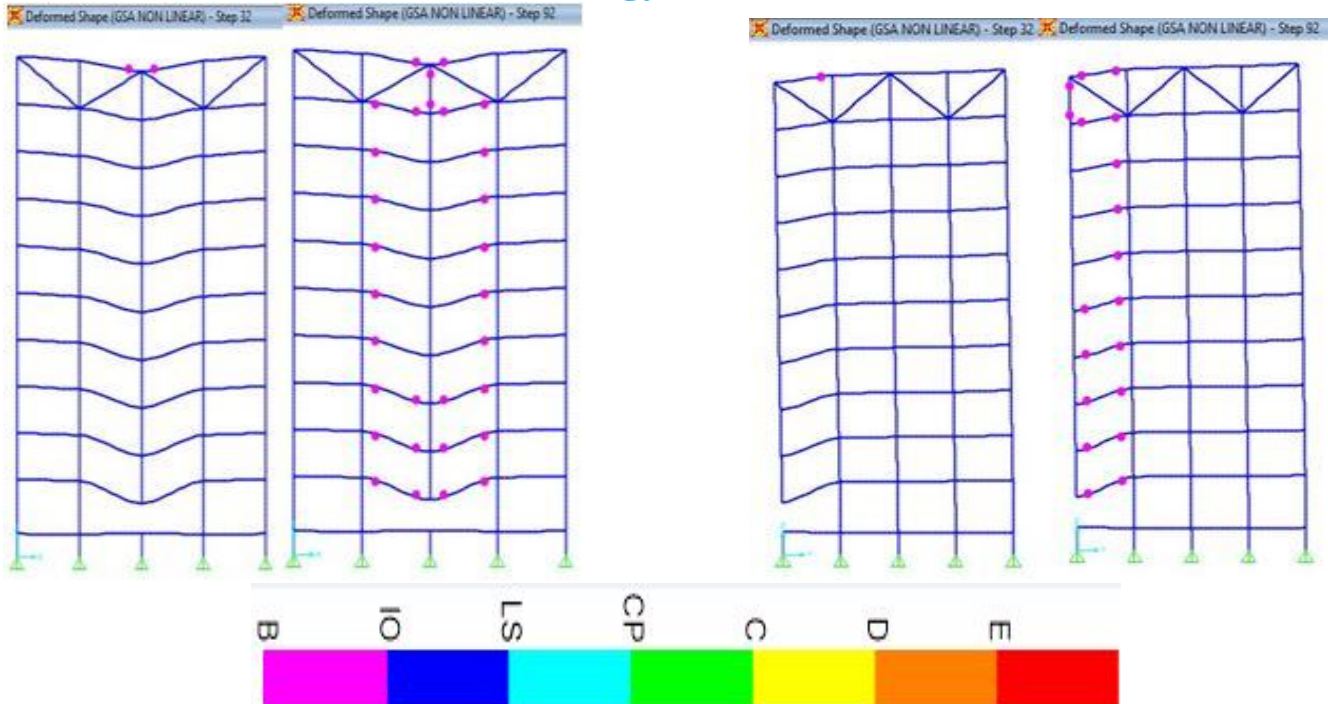
Fig. 7 Hinge formation in long bay middle column removal case after mitigation
