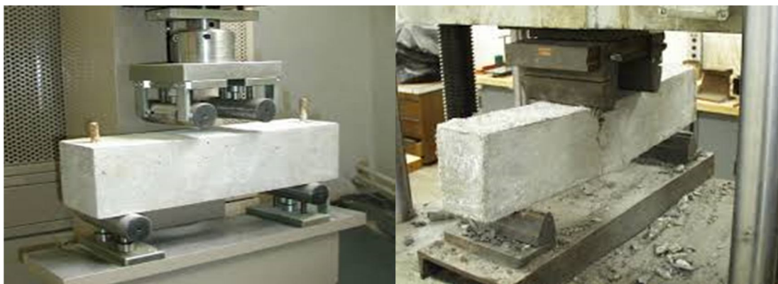
Fig 3.9 Flexural strength setup before testing
