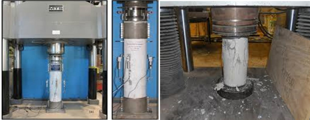
Fig 3.4 Crack pattern at ultimate failure load of cylindrical specimen
