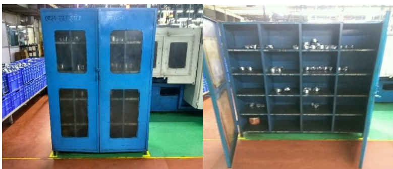
Fig.4 Setting Piston inspection almira
