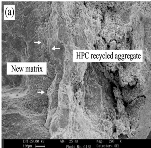
Figure-4 An image showing ITZ of newly formed matrix and HPC recycled aggregate
