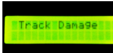
Fig.11. LCD displaying track damage detected
