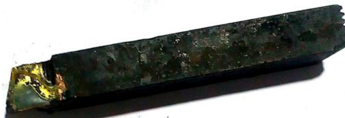
Fig. 2 A single point carbide cutting tool
