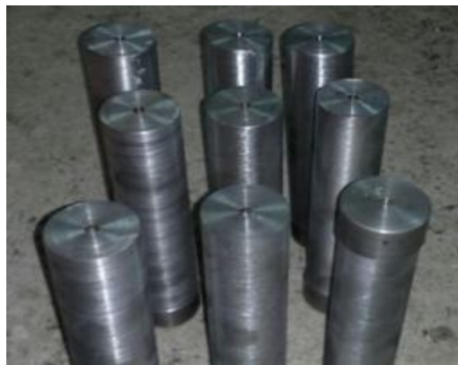
Fig. 1 After turning operation EN8 material piece
