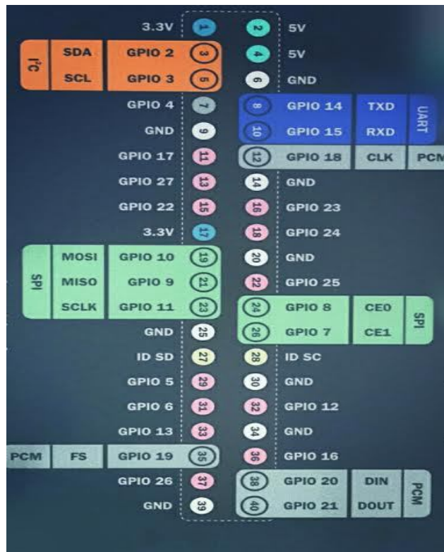
Figure 4 Pin Diagram of GPIO Pins
