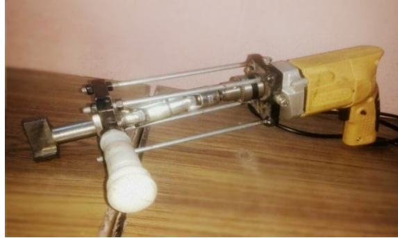
Fig.5 Experimental setup for the square hole drill machine.
