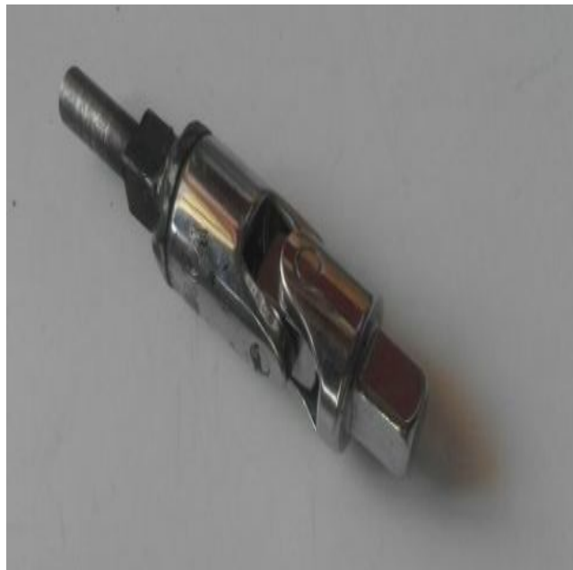
Fig.4.3 Image of universal coupling selected for the machine.
