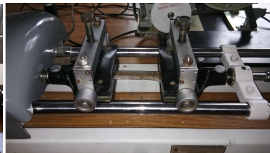
Fig.7 sample loaded in Tensometer
