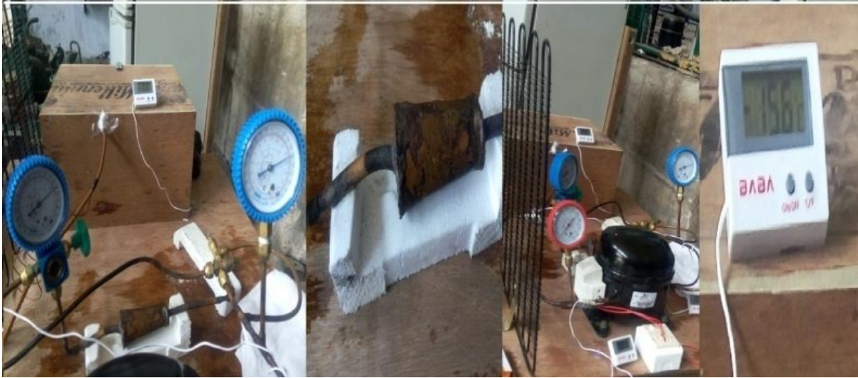
Fig 4 schematic diagram of installed setup (In above figure temperature of evaporator is -15.6^{\circ} )
