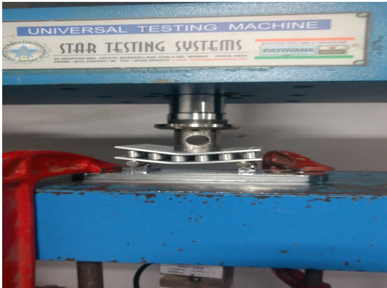
Fig.6-Bending Test on Sandwich Structure
