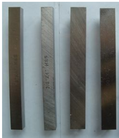
Fig. 2 Geometry of the HSS turning tools
