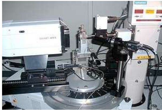
Fig .3(b). ADXRD In-house Setup
