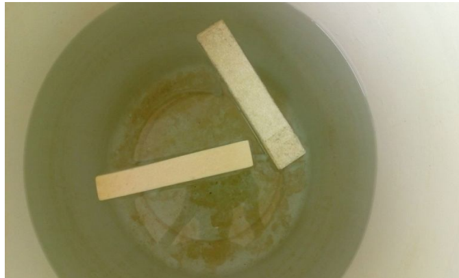
Fig 7. Specimen during water absorption test
