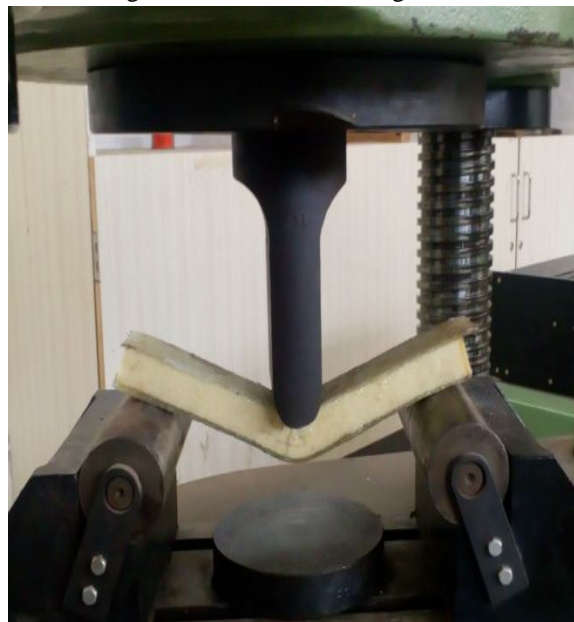
Fig 5. Specimen during bending test
