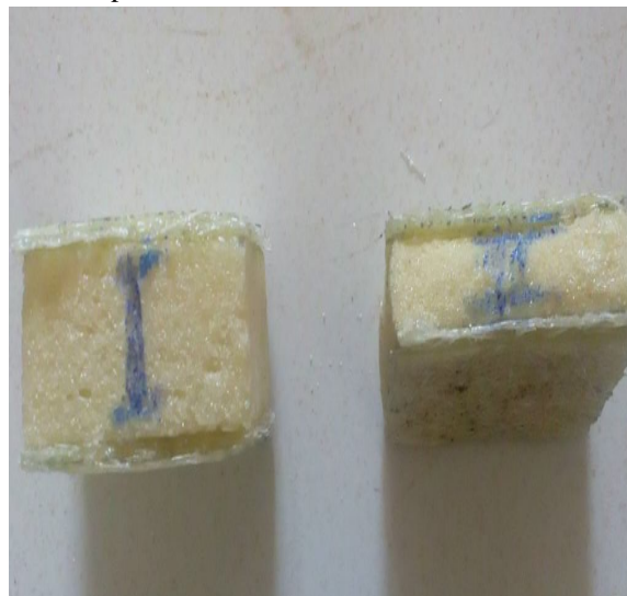
Fig 8. Specimen before & after the compression test
