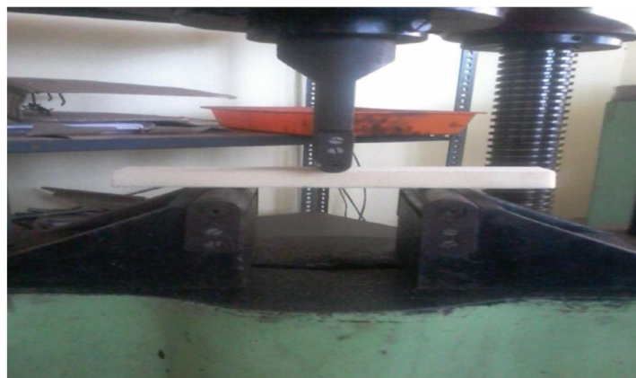
Fig 6. Specimen during bending test
