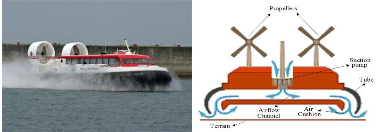
Fig. 1 A practical hover vehicle(left) and its functional description (right)
