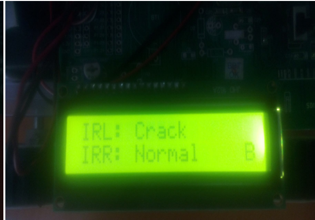
Fig 8: Left crack is detected
