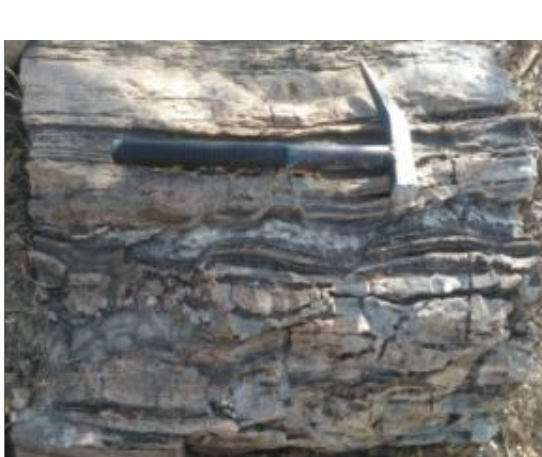
E: Bedding plane is visible by variation in colour, differential weathering and the presence of thin quartz rich layers in carbonate rock near Khiwandi area.
