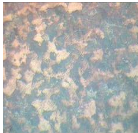
Fig 6(b) Un coating surface after testing
