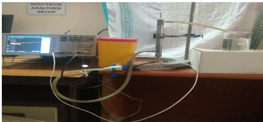
Figure I: Spectrum analyzer setup with resonator
