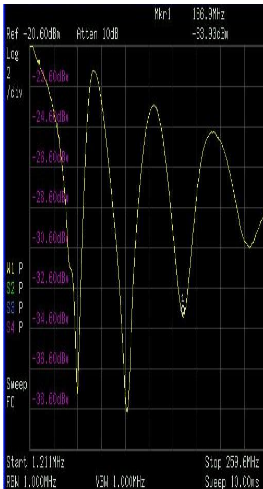
Figure (b): Resonant frequency for the third resonance is 166.9MHz.
