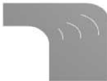
CFD model of economizer duct with curved vanes
