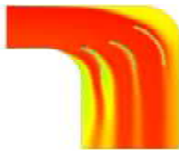
Pressure contours of economizer duct with curved inlet vanes Above figure shows the pressure contours economizer duct modification with inlet vanes fillet radius 0.5m shows lesser pressure drop reduced.
