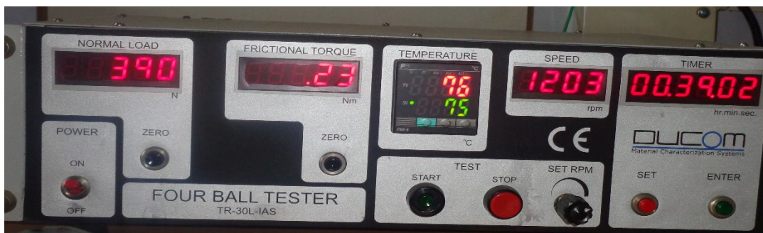
Fig. 11: ASTM D4172B conditions of tribotester.
