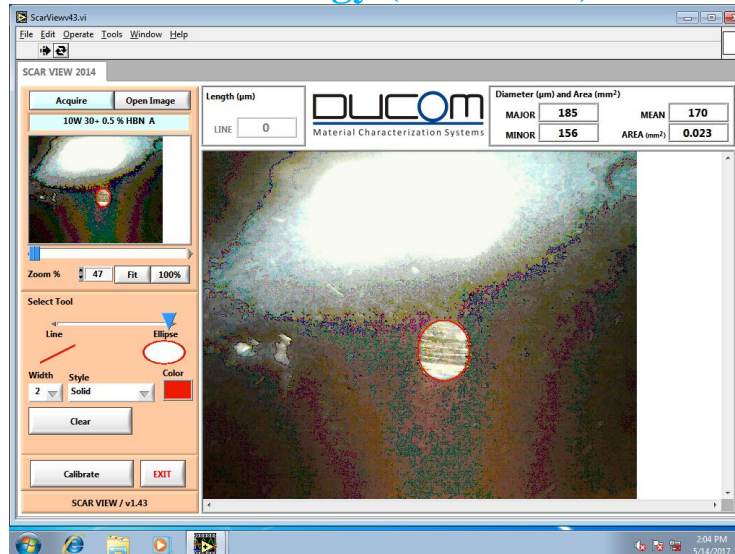
Fig 14 : SEM micrograph worn surface on SAE 10W30 +1.0 % HBN Wt ball under lubricated.
