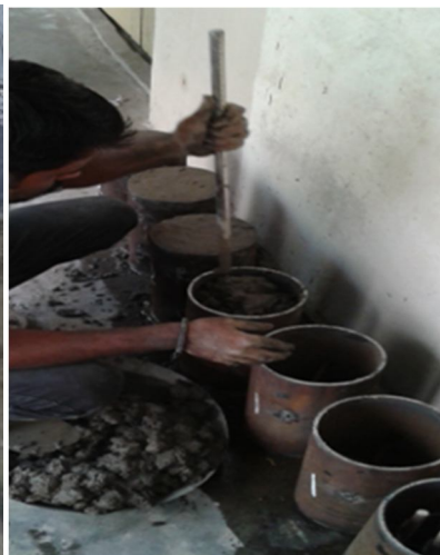
Compacted by iron rod
