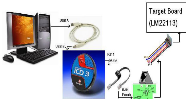
Figure 3: Software process flow & IED installation guide
